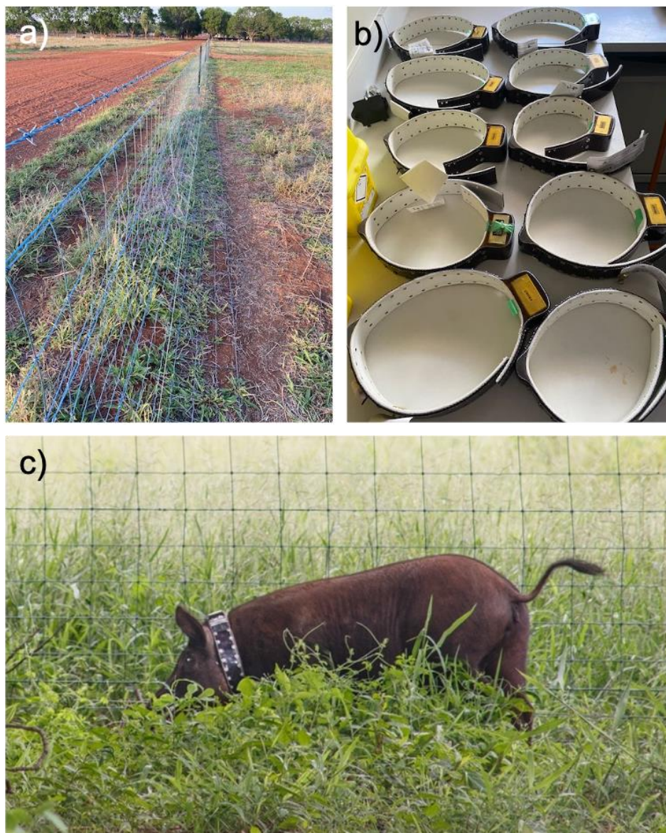
Figure 17: a) Feral pig proof fence with electric wire constructed around 23 acres of paddock and mixed woodland; b) Purpose-built feral pig collars with location fixing, ambient temperature, and body temperature recording and data-logging; c) Feral pig released inside the fenced paddock and fitted with locating and body surface temperature recording collar.
